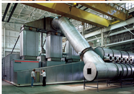
TOP: Catalytic Oxidizers are used to control VOC and HAPs from many surface coating processes.
